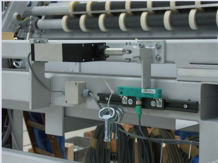
Fig. 1: PMI104-F90-IE8-V15 with a target 5 mm wide
