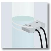
Fill level measurement of liquids
