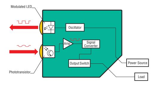
A photoelectric sensor is a device that detects a change in light intensity. Typically, this means either non-detection or detection of the sensor's emitted light source. The type of light and method by which the target is detected varies depending on the sensor.
