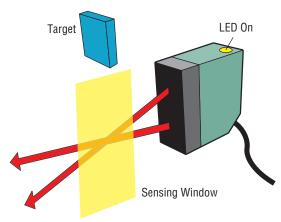
high amount of excess gain is available, which enables the sensor to easily detect narrow or low reflectivity targets.
