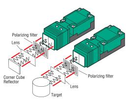
Non-polarized retro-reflective photoelectric sensors usually allow longer sensing ranges than polarized versions, but can falsely identify a shiny target as a reflector.
