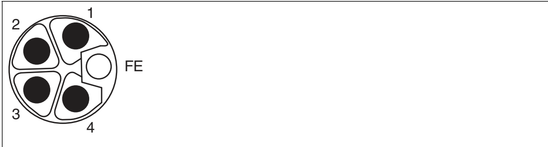
Figure 2.3 Schematic drawing of M12 L-encoding (socket); port X04 (OUT)
